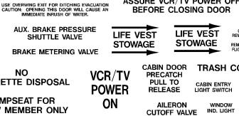
USE OVERWING EXIT FOR PRIMARY DITCHING EVACUATION CAUTION: OPENING THIS DOOR WILL CAUSE AN IMMEDIATE INRUSH OF WATER, UNLESS WATER BARRIER IS INSTALLED
