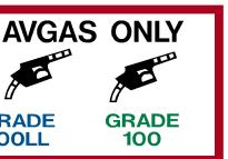
SERVICE THIS AIRPLANE WITH 100LL/100 MIN AVIATION GRADE GASOLINE. TOTAL CAPACITY 77.5 U.S. GAL.
