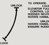
LOCK ELEVATOR FULL DOWN OR CONTROL LOCK INSTALLED RUDDER NEUTRAL ROTATE HANDLE TO LOCK UNLOCK ROTATE HANDLE TO UNLOCK ENSURE RUDDER IS FREE
